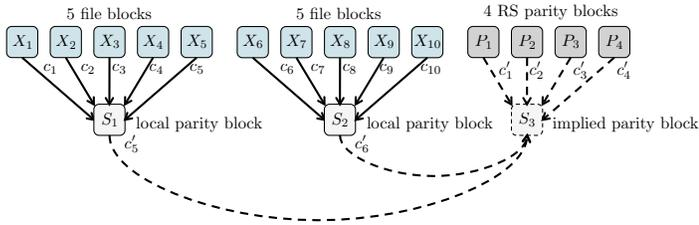
**Figure 2: Locally repairable code implemented in HDFS-Xorbas.** The four parity blocks  $P_1, P_2, P_3, P_4$  are constructed with a standard RS code and the local parities provide efficient repair in the case of single block failures. The main theoretical challenge is to choose the coefficients  $c_i$  to maximize the fault tolerance of the code.
