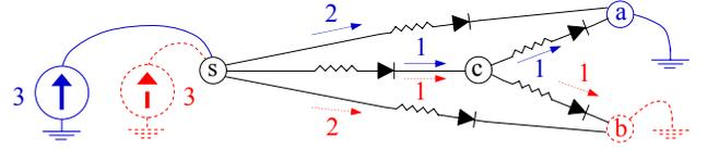
**Figure 2:** Node  $s$  injects two classes of electrical currents with intensity 3, one destined for node  $a$  and the other for node  $b$ . For all resistors  $\sigma_{ij} = 1$ , and for all edges  $\mu_{ij} = 5$ .
