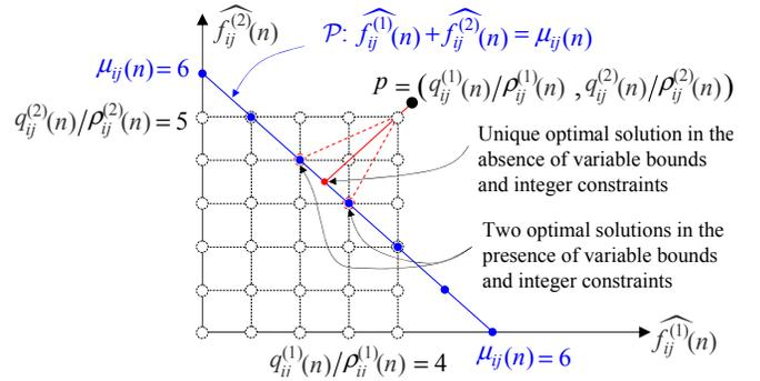
**Figure 3: Geometry of solving (25) for a two-class case when  $q_{ij}^{(1)}(n)/\rho_{ij}^{(1)}(n) + q_{ij}^{(2)}(n)/\rho_{ij}^{(2)}(n) > \mu_{ij}(n)$ .**
