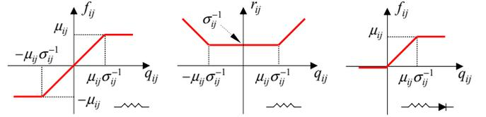
**Figure 1: The nonlinear resistive edge with an ideal diode: (left) The current-voltage curve of the resistor. (middle) The resistive-voltage curve of the resistor. (right) The current-voltage curve of the resistor and diode together.**
