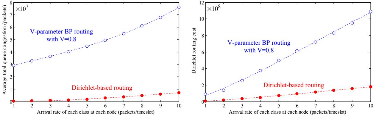
Figure 5: Expected time average total number of packets in the network against the exogenous arrival rates changing from  $\lambda = 1$  to  $\lambda = 10$ . Dashed lines display third degree polynomial interpolation.
