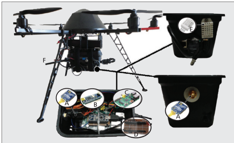
Figure 2. Our prototype has the sensor node located in the undercarriage and involves the following items: a) the ZigBee wireless communication module; b) Arduino, used to monitor the power consumption of ZigBee and UAV; c) Raspberry, the computational component of the sensor node; d) the Power Meter Shield, connected to the Arduino and assisting in monitoring the power consumption of ZigBee; e) the temperature and humidity sensors providing basic information on weather conditions; f) the antenna coupled to ZigBee.
