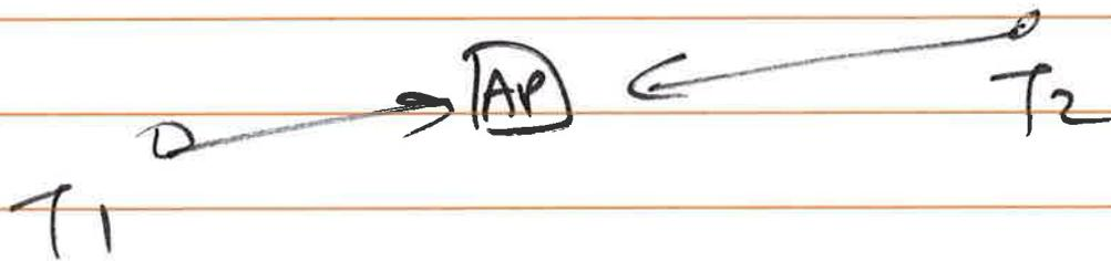
Virtual carrier sensing at the receiver is needed
