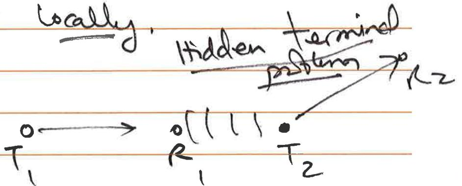
The possible interference condition at the receiver may go undetected.
