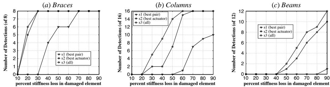
Figure 4. Performance comparison for actuator/sensor schemes as function of damage stiffness loss.
