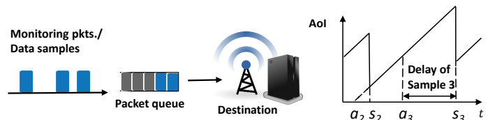
Fig. 1. A status update example with one source (sampler), one destination and a single queue to illustrate AoI, wherein a_i denotes the arrival time of a packet and s_i denotes the update time of a packet.
